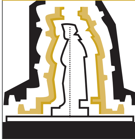
11 Demolding the skin mold
