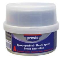
2-compontent, solvent-free epoxy fine putty for the use above water and especially underwater environment on all customary boatbuilding materials. The putty levels out slight unevennesses and fills capillary cracks. It is extremely water-resistant and scarcely shrinks. Especially recommended for the repair of osmosis damages.
