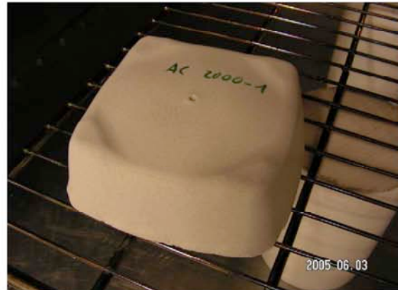
Figure 5: Aquacore specimen at 2000\text{W/m}^3
