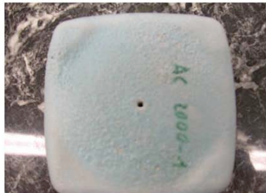
Figure 8: drying at 2000W/m³
