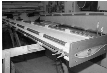
Each mould half is stiffened with two 50 mm aluminium tubes
