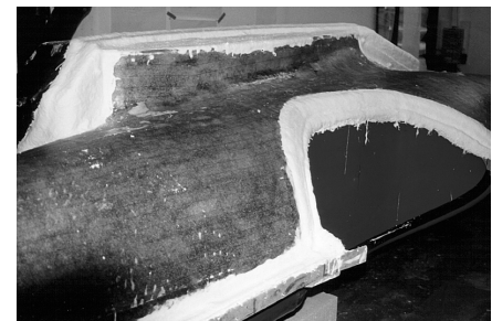
The finished edge reinforcements. A honeycomb sandwich construction was adopted for the large surfaces to reduce weight.
