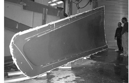
The female mould's inner side shows the smooth, glossy surface of R&G mould resin P
