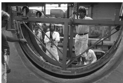
Engine cowlings for a General Electric CF 6/50 (Boeing 747, DC 10, Airbus A 300). The master pattern is lifted with a crane
