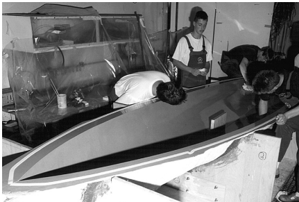
Female mould of epoxy resin / laminating ceramic
