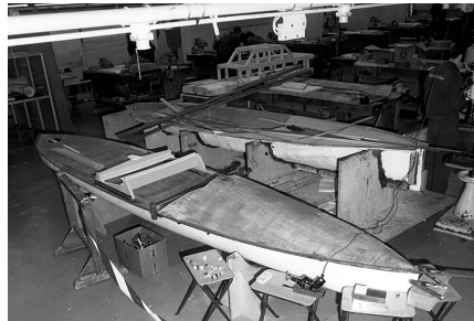
The finished hull is glued to the top panel
