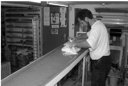
M1 glass fabric pre-impregnated with laminating ceramic is laid on the wet epoxy resin / glass fabric laminate
