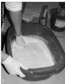
The laminating ceramic is mixed (0.28 l water to 1 kg powder)
