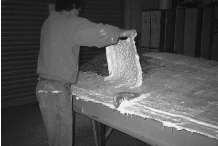
An M1 fabric layer pre-impregnated with laminating ceramic is laid on the "wet" epoxy resin laminate
