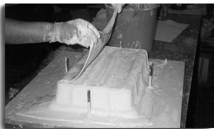
Making of a female mould for a receptacle
