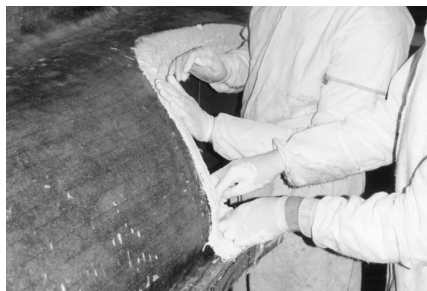
The edge reinforcements are laminated
