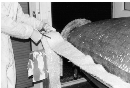
M1 glass fabric is measured and cut to size
