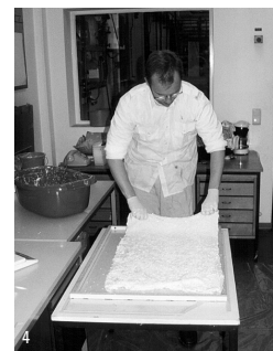
... the M1 fabric is laid on the "wet" epoxy resin laminate ...
